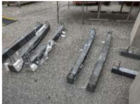
Fig. 5 Curved UHPC beams after form removal
