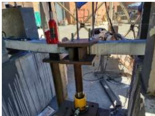
Fig. 7 Second test of a UHPC beam
