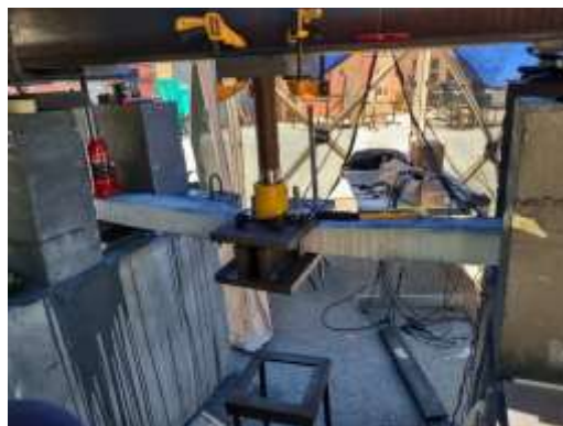
Fig. 6 First test of a UHPC beam
